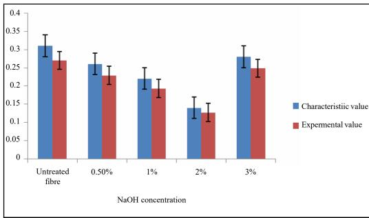
Fig. 2: Characteristic and experimental values of breaking strength of banana fibres treated with NaOH by the Weibull model
