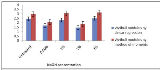
Fig. 4: Weibull Modulus by Linear regression and Method of moments for the breaking strength of banana fibres treated with NaOH
