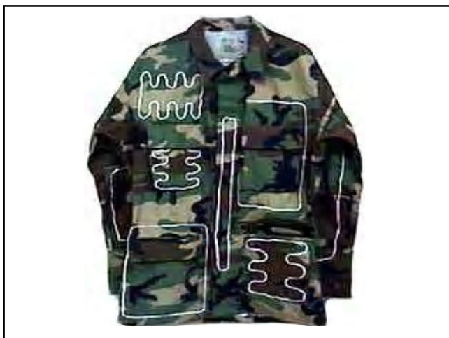
Fig. 10 : Army cloth with integrated communication antenna
