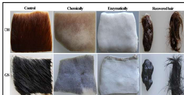
Fig. 8 : Dehairing effect by conventional chemical treatment versus enzymatic method (Zhou et al. , 2022)
