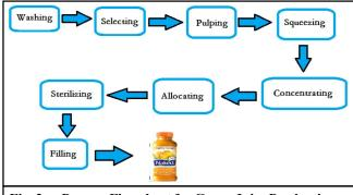
Fig. 2: Process Flowchart for Grape Juice Production
